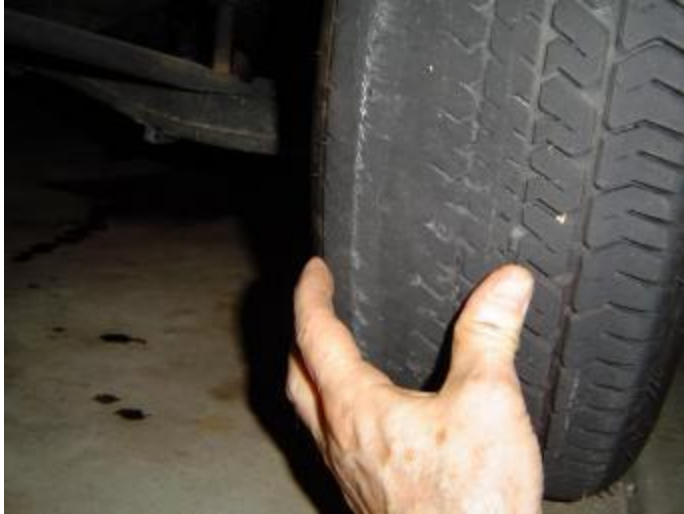
Uneven wear on the inner area of the tread caused by toe-out misalignment.
