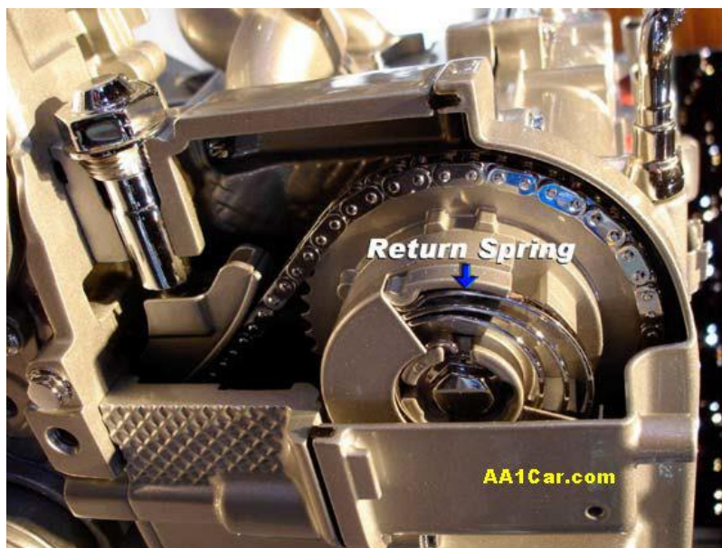
A circular spring in a helical gear phaser returns the cam back to its original base timing position when oil pressure is relieved.
