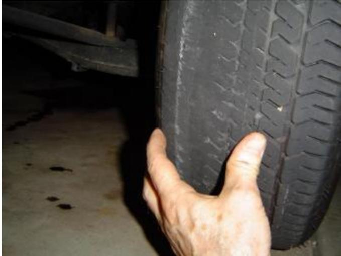
*Severe tread wear caused by misalignment.*
