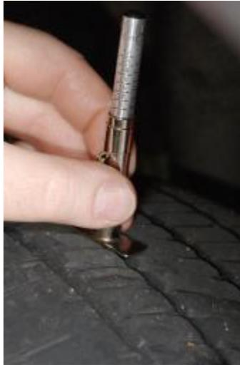
*Tire tread wear can be measured with a simple gauge like this. Tread depth should be checked in the middle of the tread, and in about one inch from each side of the tread.*
