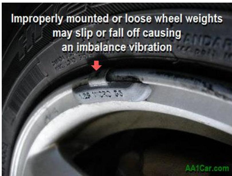
*Clamp-on tire weights that are not properly mounted may come loose and create an imbalance that causes a vibration.*
