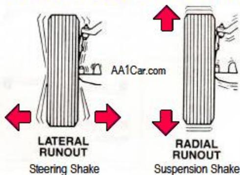
*Radial or Lateral Runout can cause tire vibrations*
