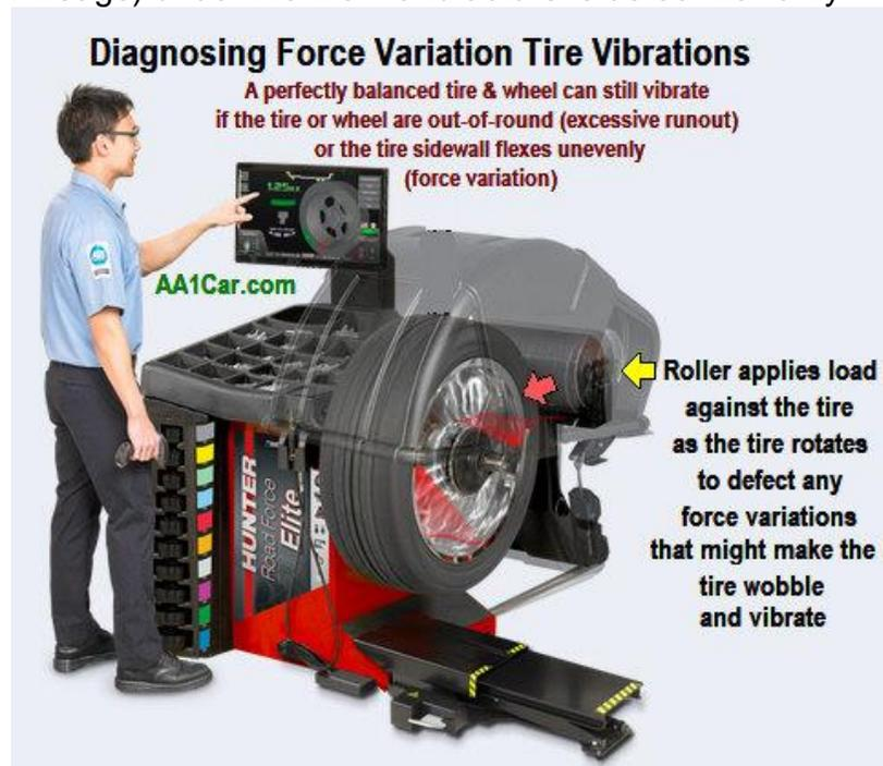
*This Hunter Road Force Elite tire balancing machine uses a roller to detect force*
