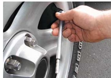
c) Press the tire gauge straight and firmly until the scale extends.
