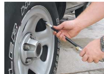
d) If needed, add air and recheck pressure with the tire gauge.
