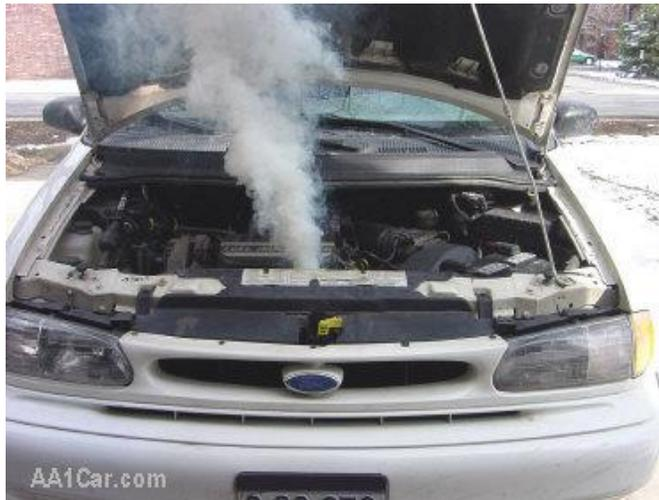
Is your engine overheating? Most engines are designed to operate within a "normal" temperature range of about 195 to 220 degrees F. A relatively constant operating temperature is essential for proper emissions control, good fuel economy and performance. But problems can arise that cause the engine to run hotter than normal, resulting in engine overheating.
