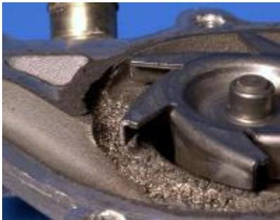
*Cavitation damage inside a water pump*
