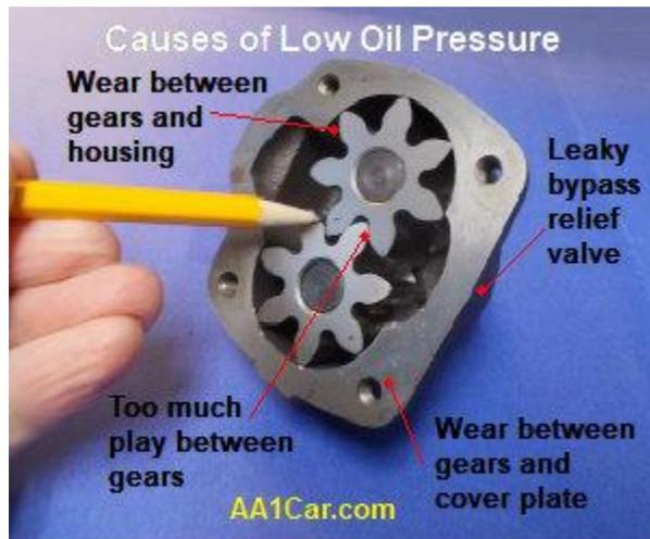
*Internal pump wear and leaks can cause a loss of oil pressure.*
