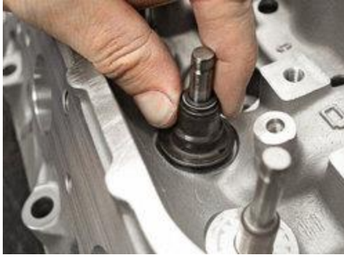
Valve guide seals fit around the valve stems on top of the cylinder head.
