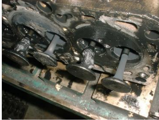
Heavy carbon deposits on the valves are caused by worn valve guides and seals.
