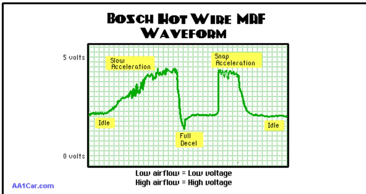
Like throttle position sensors, there should be smooth linear transition in sensor output throughout the rpm range. If the readings jump all over the place, the computer won't be able to deliver the right air/fuel mixture and driveability and emissions will suffer. So you
