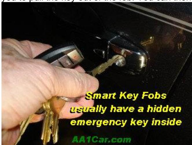
If the door handle does not have an obvious keyhole to accept the emergency key or a valet key, there is usually a "hidden" key slot under the handle trim near the edge of the door. You may see a small slot in the bottom of the handle trim. Insert the key into this slot to pry the trim cover off. Some covers slide up to remove, or to the right to remove. Once the cover is off, you should see the key slot for the emergency key to unlock the door.
