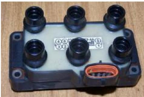
*Ford DIS V6 ignition coil. Note terminals are in coil wiring connector.*
