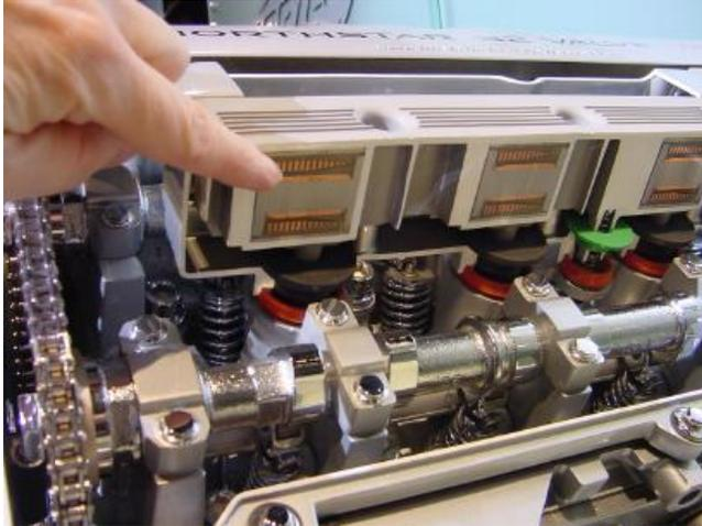
*Cutaway of coil-on-plug ignition on a Cadillac Northstar engine.*
