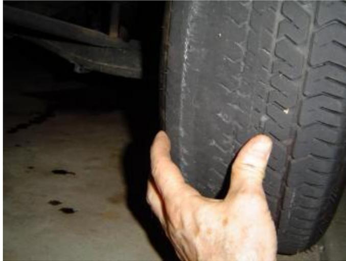
*Inside shoulder wear like this on both front tires indicates toe misalignment.
