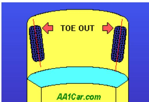
*A toe-out condition is the most common cause of toe wear on front tires.*
