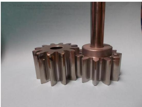
*Here you can see the difference in the length of the drive and driven gears.*
