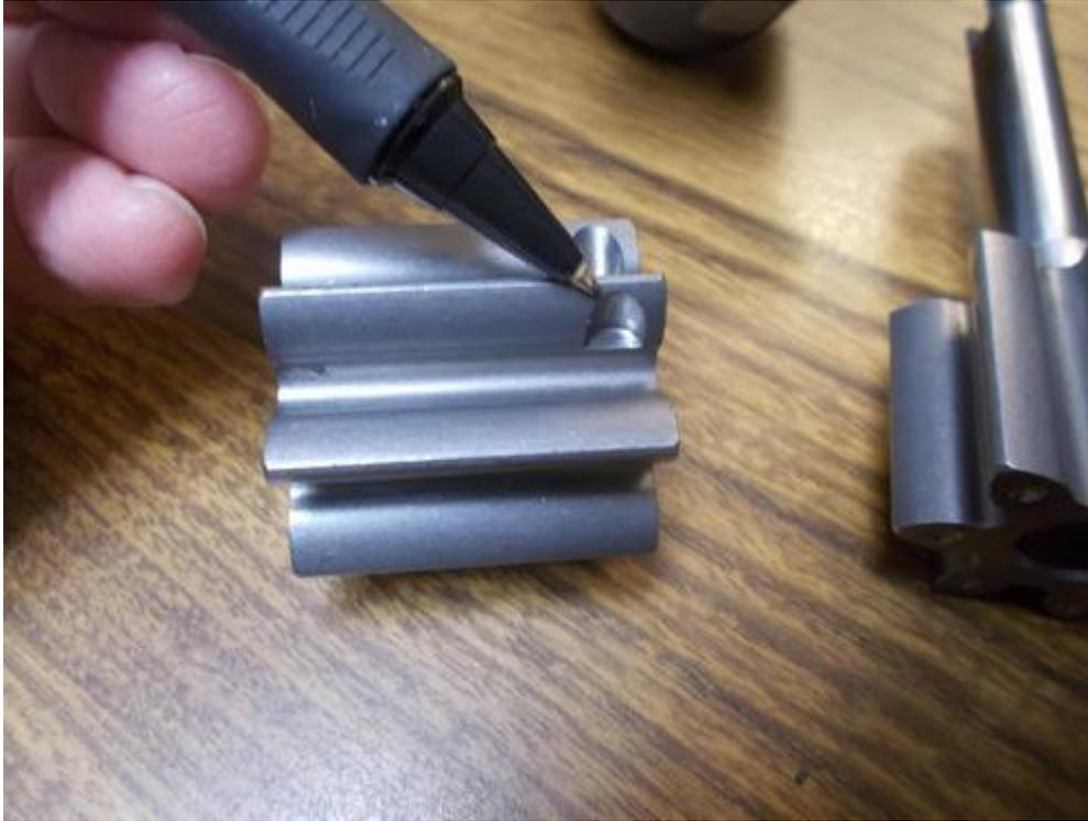
*Small scallops machined into the face of each gear tooth on the driven gear gives oil an extra push as it reaches the pump outlet port.*
