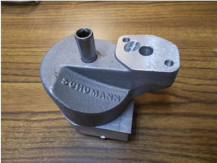
*The pump housing in the Gear rotor design is offset to one side so the design will work. This requires a modified oil pan and relocated pickup tube.*
