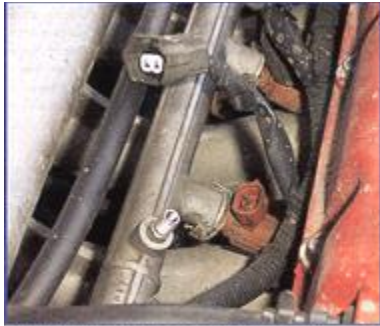
The fuel injection pressure test port on the fuel rail of a 2000 Kia Sephia
