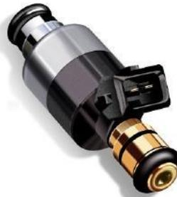
*On most EFI systems, voltage is supplied directly to the injectors and the PCM energizes the injector by grounding the circuit.*
