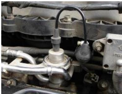
*The fuel pressure regulator is usually mounted on the fuel rail that supplies the injectors.*
