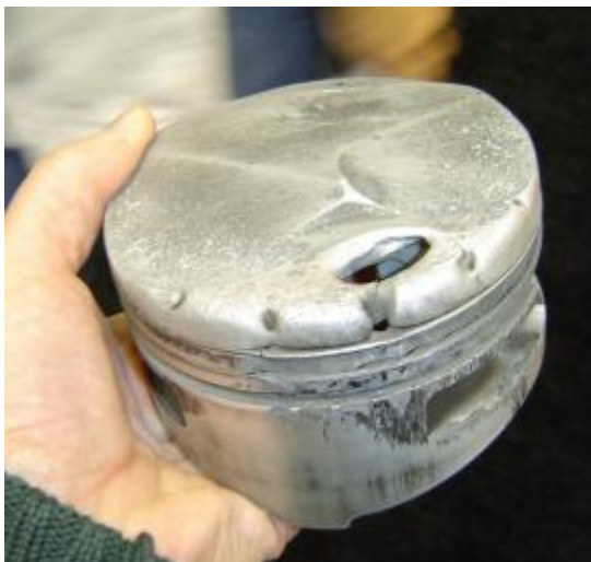
Detonation damage to a piston
