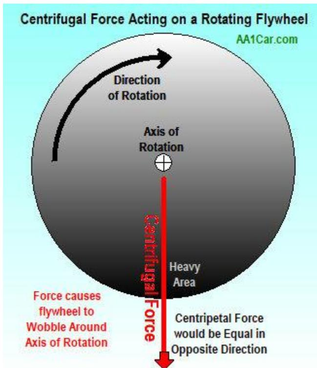
Centrifugal force equals the mass of the spinning object (or the heavy spot on a crank or flywheel) times the speed of rotation squared divided by the radius or distance from the axis of rotation.
