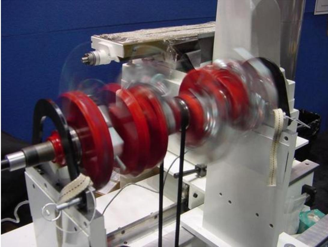
*The crankshaft is then spun while sensors on the balancing machine detect vibrations. The software in the balancer calculates where the imbalance is and how much it is so corrections can be made. A second spin after corrections have been made will verify the crank is balanced.*
