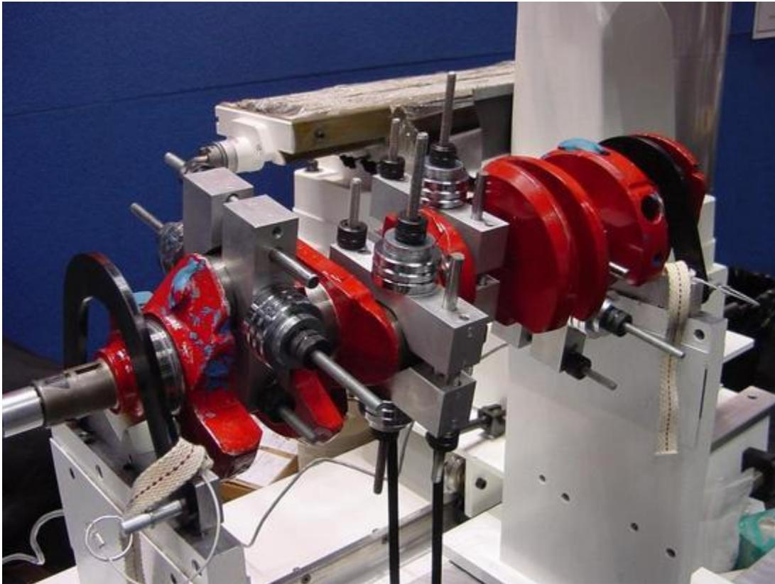
*Bobweights that equal the reciprocating weight of the upper rods and pistons are assembled and mounted on the crankshaft rod journals.*
