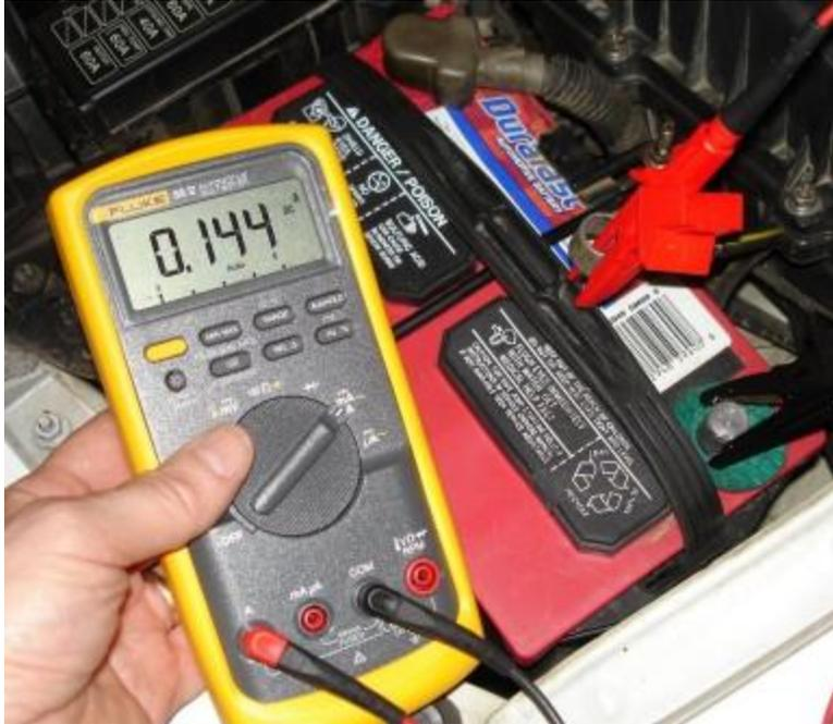
*Measuring current draw with a multimeter.
