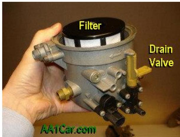
*An important part of diesel maintenance is draining water from the fuel filter housing periodically.*
