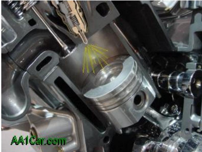
*Fuel is injected directly into the combustion chamber under high pressure. Pressure leaks in the high pressure pump, fuel circuit or injectors can cause hard starting and misfire problems.*
