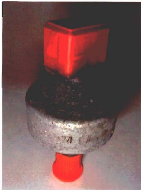
Figure 16. SCDS with melted base.
