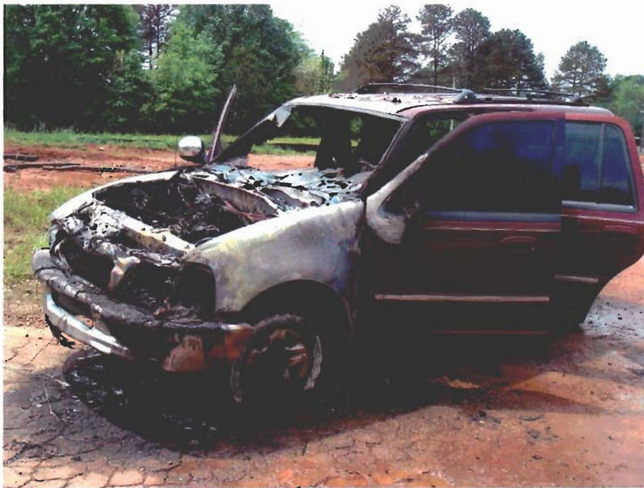
Figure 17. Burns Patterns On Test Vehicle.
