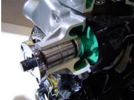
A worn seal on the water pump shaft can leak coolant.
