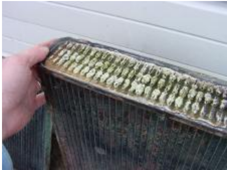
This radiator is badly corroded and is not worth fixing
