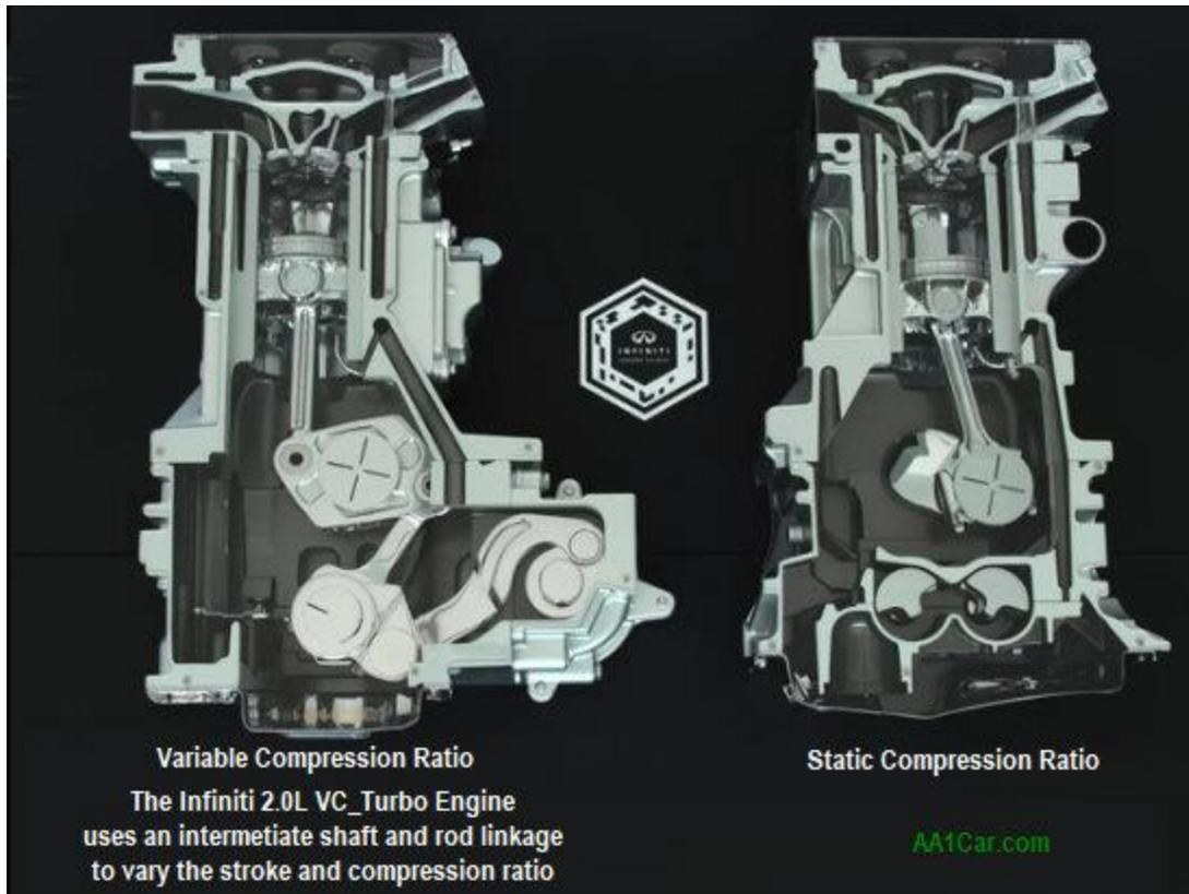
Some engines even have a Variable Compression Ratio, such as the Infiniti 2.0L VC\_Turbo engine. The engine has an intermediate shaft that changes the rod linkage to vary the compression ratio. A higher compression ratio is used to maximize fuel economy. The compression ratio is then decreased when the turbocharger is delivering boost to optimize power.
