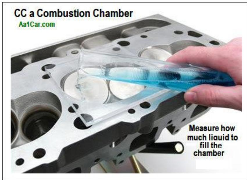
Combustion Chamber Volume is difficult to measure directly because of the complex shape of most combustion chambers. So chamber volume has to be measured by filling the chamber with liquid (water or a light oil) and measuring how many CC's (cubic centimeters) of liquid it takes to fill the chamber. A plastic plate is used to cover the chamber and the liquid is poured in through a small vent hole. NOTE: The valves and spark plug must be installed to contain the liquid.
