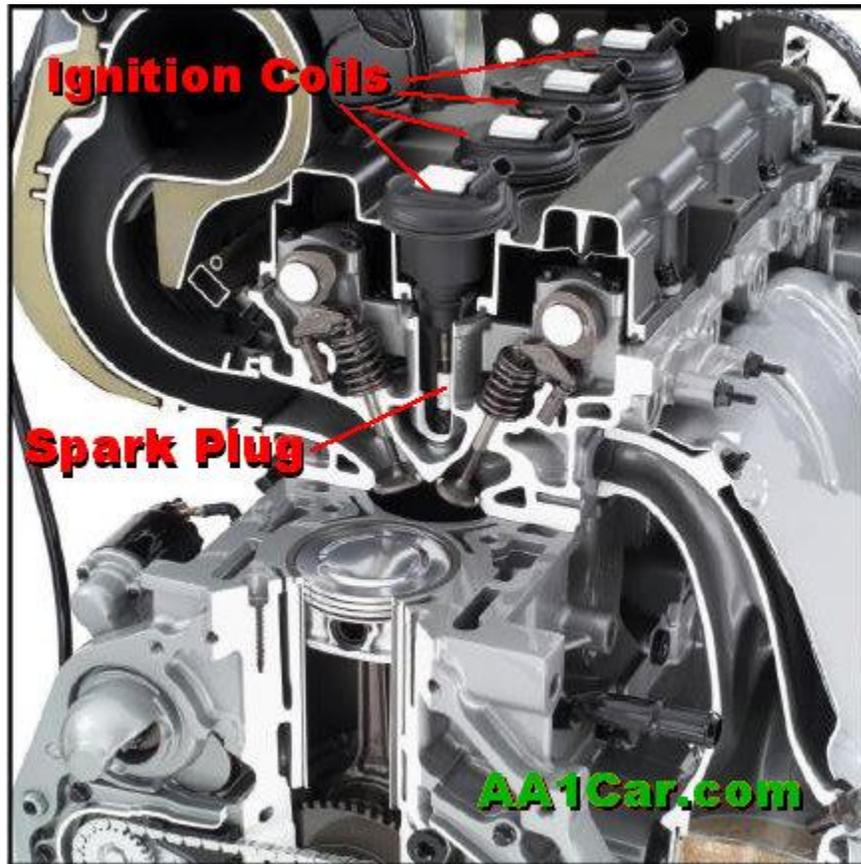
*Coil-On-Plug ignition system on a General Motors Vortec 3500 engine.*
