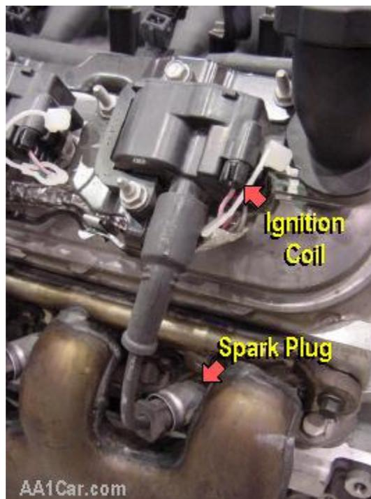
*A Coil-Near-Plug ignition system on a General Motors LS V8.*
