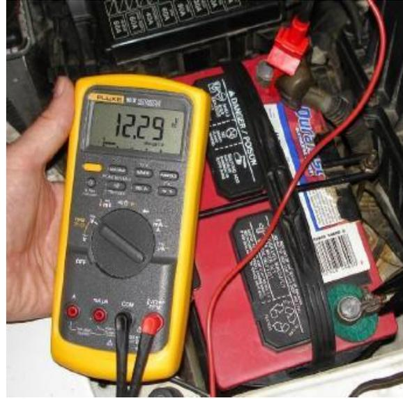
*The left photo shows normal alternator charging voltage with the engine idling. The photo at the right shows low charging voltage with the engine idling. A low reading tells you the charging system is not generating enough voltage to keep the battery charged or to meet the vehicle's electrical needs.*
