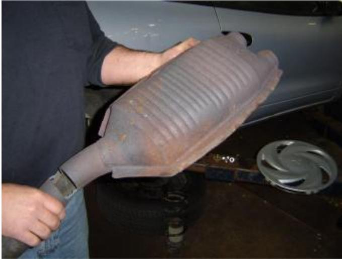
*Converters do a fantastic job of cleaning up exhaust emissions. If yours has failed, it is illegal to replace it with a straight pipe. Replace it with a new aftermarket or OEM converter.*
