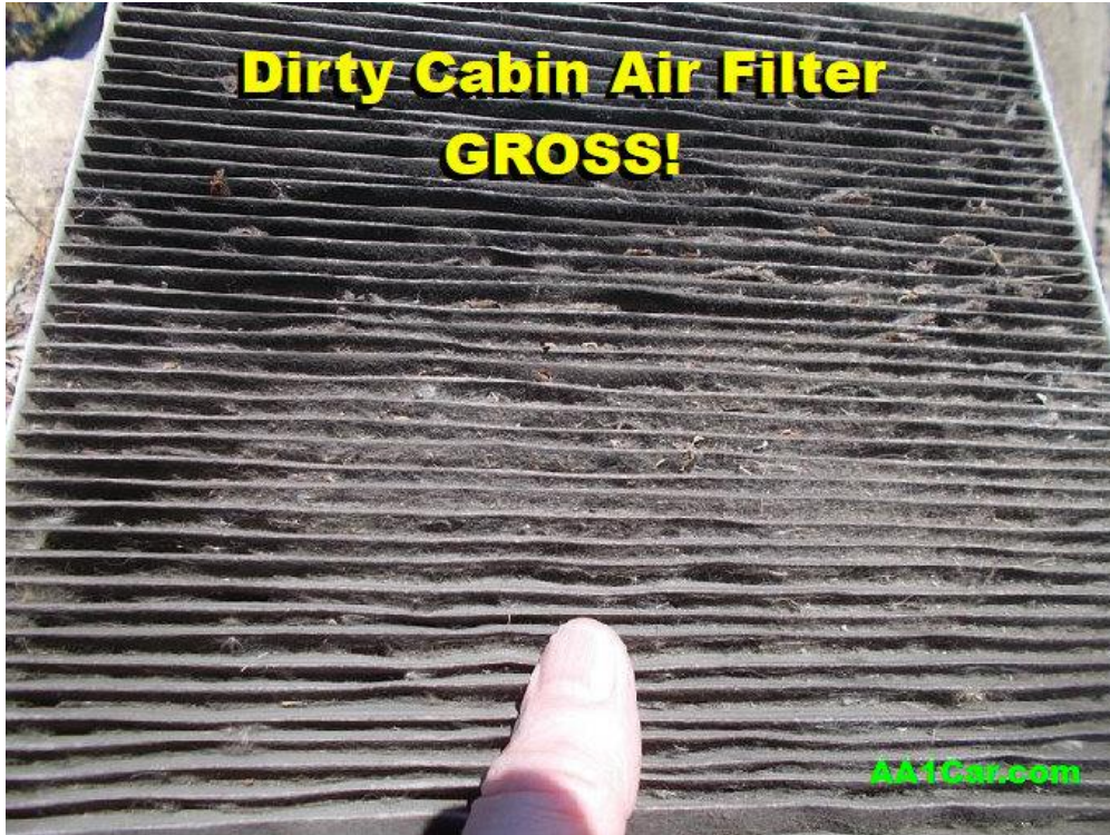
This is what a really dirty cabin air filter looks like. This one had not been changed in 8 years! The filter was so dirty that it was obstructing airflow through the heater and A/C.
