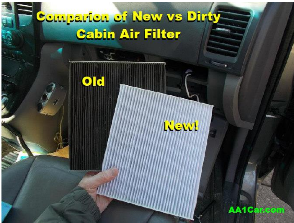
You can see how dirty the old filter is in comparison to the new filter.
