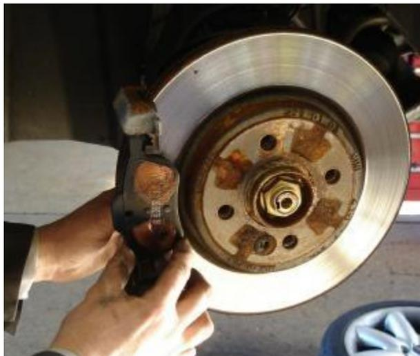
*Replacing your old noisy brake pads with ceramic pads can eliminate annoying brake squeal. Applying a moly-based high temperature brake grease to the backs of the pads can also help dampen vibrations and noise.*
