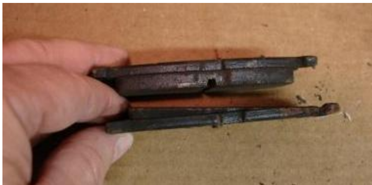
Uneven pad wear can be caused by sticking calipers slides or pistons
