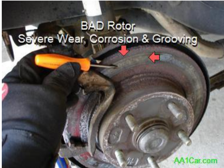
This rotor has reached the end of the road and needs to be replaced with a new one.
