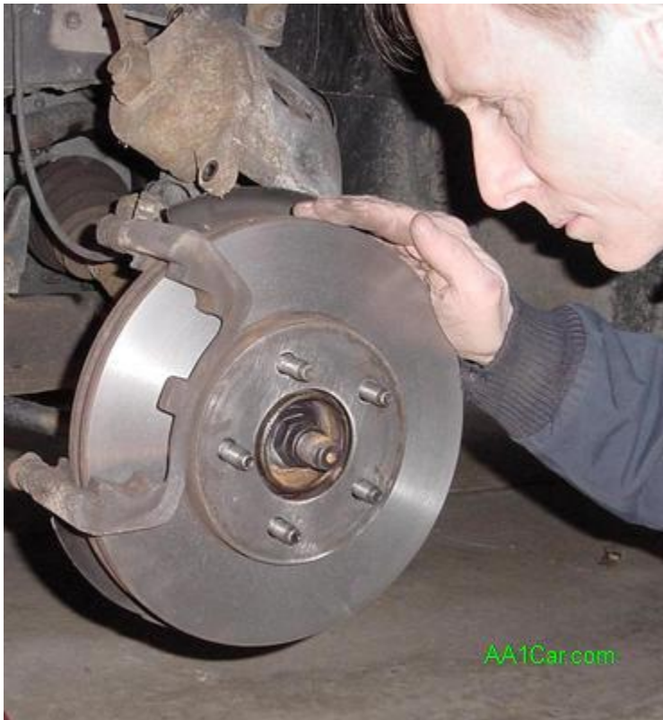
This rotor shows almost no wear and can be safely reused.
