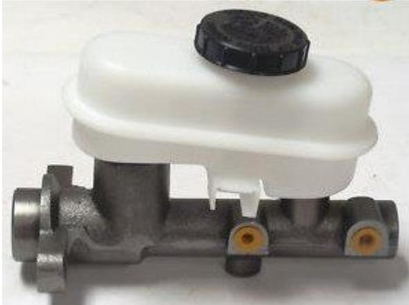
*New master cylinders may not come with a new brake fluid reservoir. If no reservoir is included, you will have to swap the old reservoir to the new master cylinder. Clean it before reusing it!*
