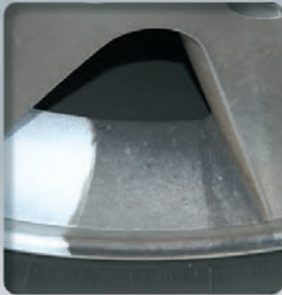
BLACK BRAKE PAD DUST Excessive wear of semi-metallic pads and rotors
