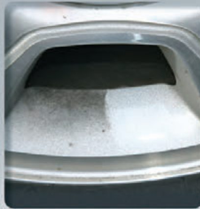
TAN BRAKE PAD DUST Excessive wear of ceramic pads
