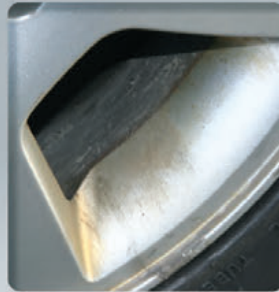
RUST BRAKE ROTOR OR PAD DUST Ferrous metal in brake dust from rotors and / or pads oxidizes on wheels, causing wheel finish to be rust-colored
