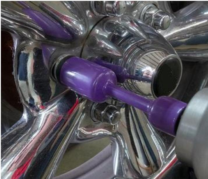
*A torque stick limits peak torque applied to a lug nut with an impact wrench.*
