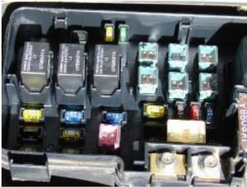
*Remove fuses and relays one at a time to find circuit that is draining the battery. Or, use a voltmeter to check for a voltage drop across each fuse. A voltage drop reading would indicate current flow in the circuit.*
