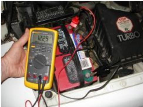
*Checking base battery voltage with a voltmeter.*
