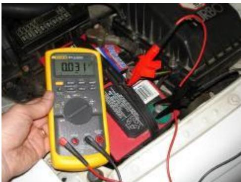
*Key-Off current drain should be less than 50 mA after 1 hour.*
