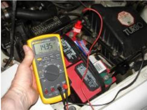
*Charging voltage with engine idling should be 13.5 to 14.5 volts.*
