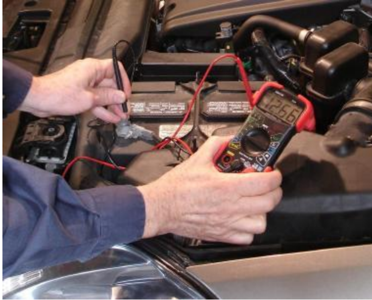
Measuring battery voltage with a digital voltmeter.
