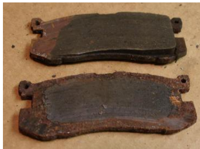
These brake pads are completely worn out!
