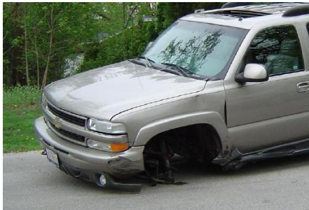
Wheel fell off after wheel bearing failed!
