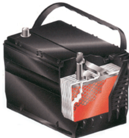
Gel-type batteries don't use liquid electrolytes and can't spill. Even so, they wear out the same as liquid lead-acid batteries. Testing is essentially the same.
