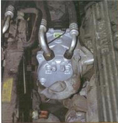
*Don't replace the compressor until you've ruled out other possibilities for poor cooling.*
