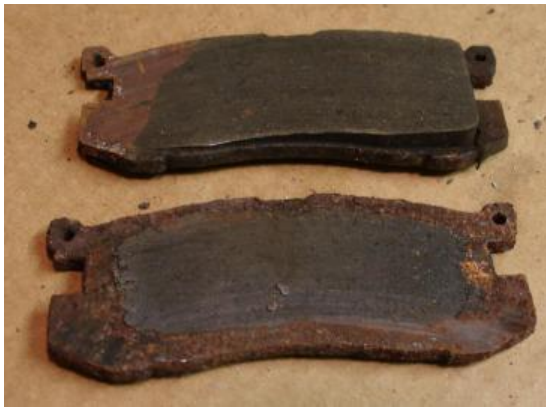
Worn brake pads are dangerous!
